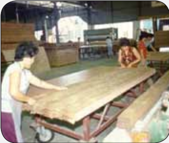
Lamination with Acrylate glue
