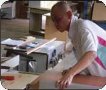
Lamination with Acrylate glue
